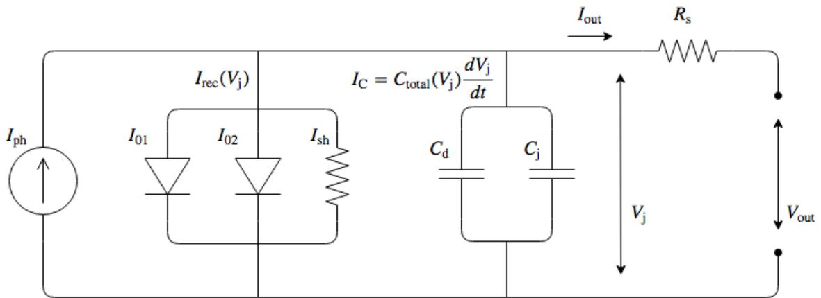
Figure 2: Equivalent circuit of a high-efficiency solar cell. Capacitors parallel to the recombination diodes are included to take charge storage in the solar cell or module into account.
