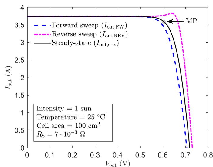
Figure 1: IV-curves simulated using the PC1D software with model parameters corresponding to a high-efficiency solar cell with an open-circuit voltage of  $\sim 0.72$  V. An output voltage sweep length of 20 ms was applied both in the forward direction (from short- to open-circuit) and in the reverse direction. Further, a steady-state IV-curve was simulated using a very long sweep duration.
