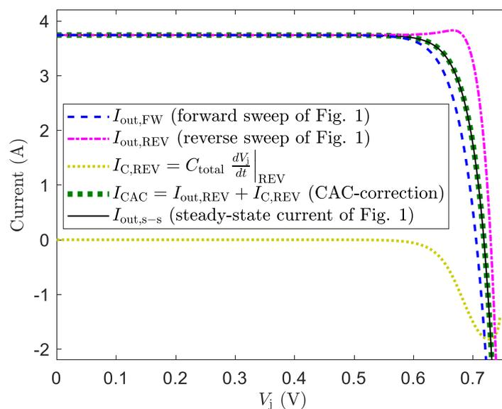
Figure 3: IV-curves of Fig. 1 with output voltages  $V_{out}$  converted into junction voltages  $V_j$ . The Capacitance Compensation (CAC) method was applied to obtain  $I_{C,REV}(V_j)$ , and consequently the CAC-corrected current,  $I_{CAC}$ , was calculated. The coincidence of  $I_{CAC}$  with  $I_{out,s-s}$  means that the CAC-corrected current is free from transient artefacts.
