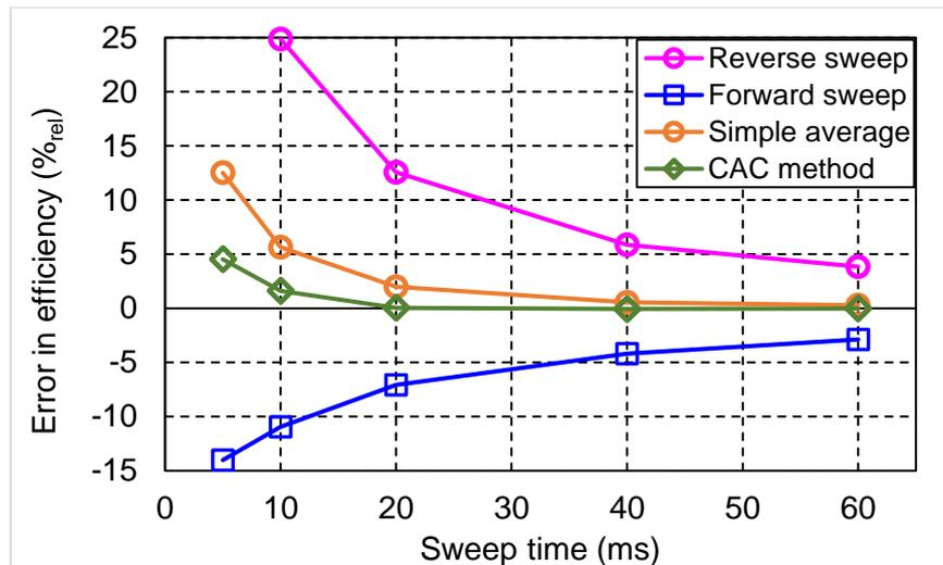
Figure 4: Relative deviation of the solar cell efficiency (in %<sub>rel</sub>) from the steady-state efficiency at different  $V_{out}$  sweep times. Forward- and reverse-swept IV-curves were utilized to calculate the efficiency both from the CAC-corrected current and from  $V_{out}$  point-wise averaged IV-curves (simple average).
